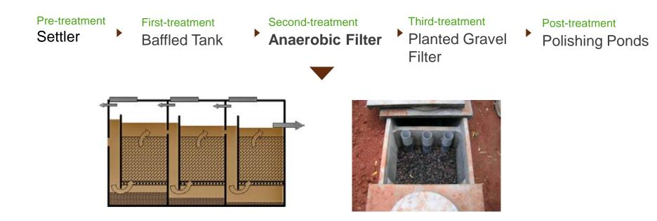
Effluent moves through filter material (cinder) from top to bottom
